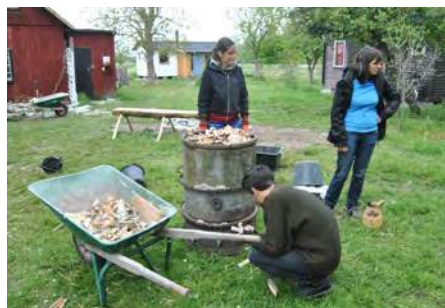
Preparing the pyrolysis process to produce biochar from residual wood. Photo by Jesús Pacheco Justo.
